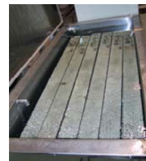
Fig. 3 The accelerated exposure situation at the water tank
